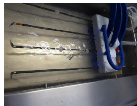
Fig. 1: (Pre-)lavado de Instrumentos robóticos en aparato de ultrasonido UniSonic® (Pre-)cleaning of robotic instruments in the ultrasound appliance UniSonic®
