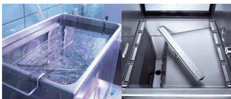
Fig. 1: Left: Ultrasound bath. Right: Interior of a washer disinfector (WD), detail spray arm.
