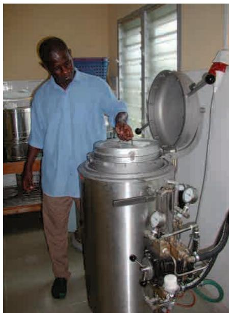
Fig. 2, page 6: Second generation prototype of the autoclave as installed in a district hospital in Eikwe, Ghana.
