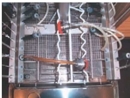
Fig. 6: Dummy plugs in positions adjacent to the logger connections
