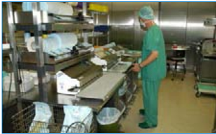
Fig. 1: Validatable heat sealer in action (here: hawo hm 3010 DC-V)
