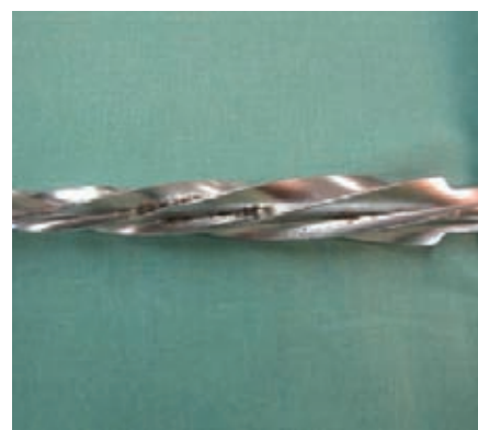
Fig. 1a/b: Typical residual contamination after inadequate reprocessing
