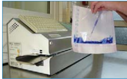
Fig. 2: Checking the quality criteria using the ink test (here: hawo InkTest)
