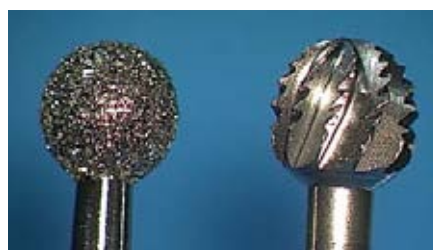
Fig. 1: Drills: diamond bur on the left, round/rose bur with A-toothing on the right, each new/unused
