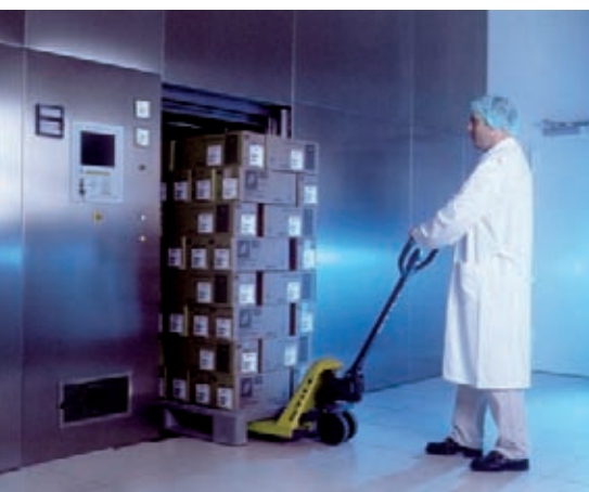
Fig. 1: Loading an EO sterilizer (closed system)
