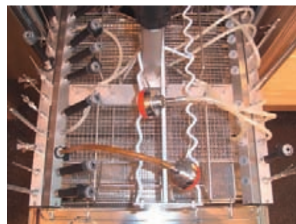
Fig. 7: On the right, oblique nozzle row with unoccupied and unconnected silicone fittings
