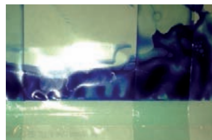
Fig. 3: Perfect seal seam (here: gusseted pouch sealed using hawo sealing device, test with hawo InkTest)
