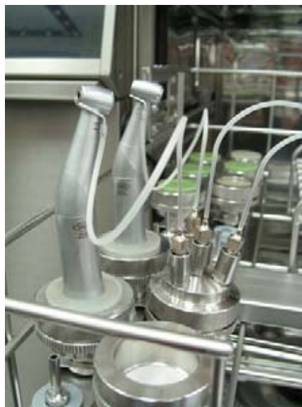
Cleaning must «get to the point» – in this case a dental handpiece, whose channels must be rinsed to be freed from residues
