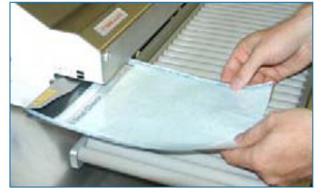
Fig. 3: Checking the sealing seam with a seal indicator (here: hawo Seal Check)
