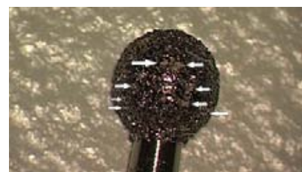
Fig. 2: Diamant 2 after mechanical cleaning (Komet cleaned with special brush, arrows point to osseous matter)
