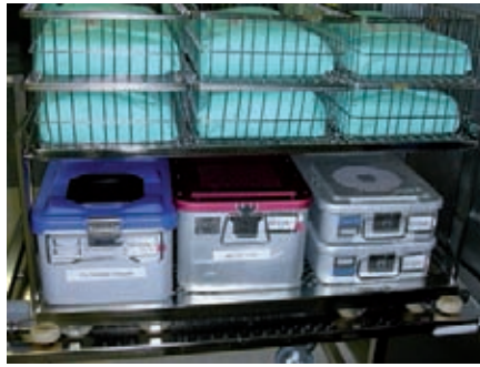
Fig. 6: Residual moisture and possible damage can be assessed from all sides.
