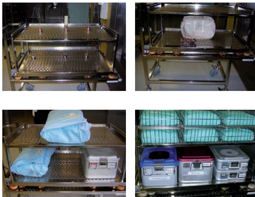
Fig. 3: Examples of sterilization processes top left to right: empty charge, BD test standard test package; bottom left to right: part load, full load
