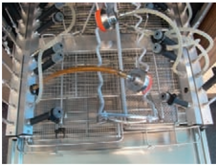
Fig. 3: Loading trolley with missing silicone fitting on right, front, and connected pressure loggers
