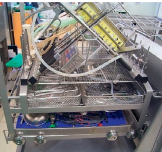
Fig. 2: Incorrectly loaded MIS injector trolley, e. g. spray shadowing due to silicone mat
