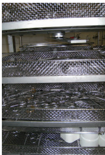
Fig. 1: Free access to the baskets, spray arm rotating freely
