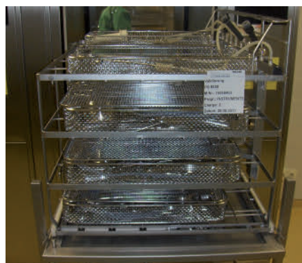
Fig. 1 and 2: Reference loads tested at validation with obvious underloading compared with actual routine loads
