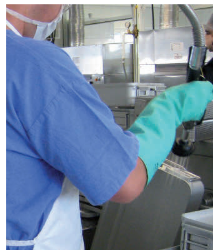
Faucet for manual pre-cleaning – with splash guard and personal protective equipment
