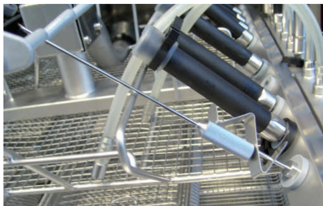
Correct connection of hollow instruments (here: Veress canula), unused sockets are closed
