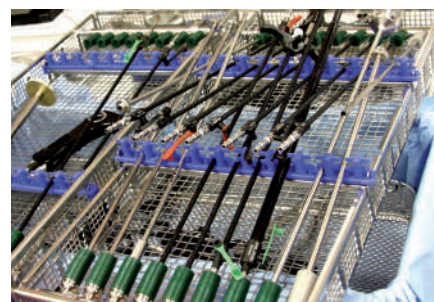
Different load carriers and different configurations of loads may lead to different qualities of cleaning results (see our draft proposal for ISO 15883 in the German mirror committee of DIN 2009) (top: Miele, Steelco, Getinge [left to right], bottom: Getinge, Belimed, Webeco [left to right])
