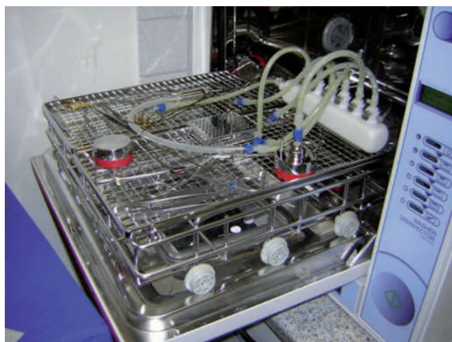
Fig. 3: Thorough flushing by complete connection, parameter control by data loggers
