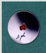
Fig. 4: Quantity of organic matter detected on instruments - equivalent blood on penny-sized plate
