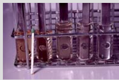
Fig. 5: Different blood concentrations and colors on metal test plates to determine recovery rates
