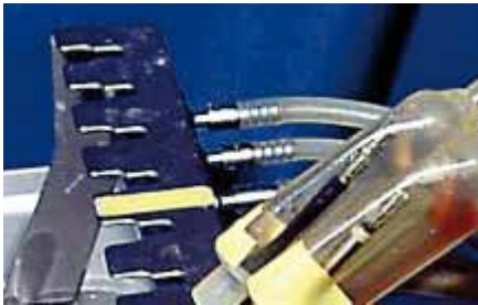
“ex juvantibus” experimental design – Demonstration of a cleaning problem in non-dismantable surgical devices, using a very basic approach
